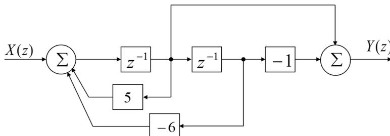
串联模拟:  $H(z) = \frac{z-1}{z^2-5z+6} = \frac{z-1}{z-2} \cdot \frac{1}{z-3}$
