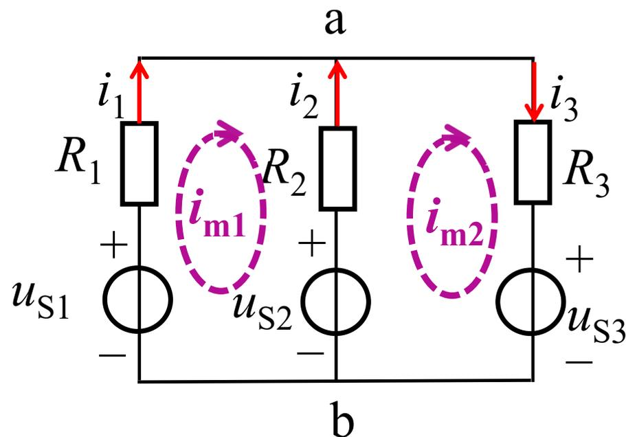
网孔1:  $R_1 i_{m1} + R_2 (i_{m1} - i_{m2}) - u_{S1} + u_{S2} = 0$
