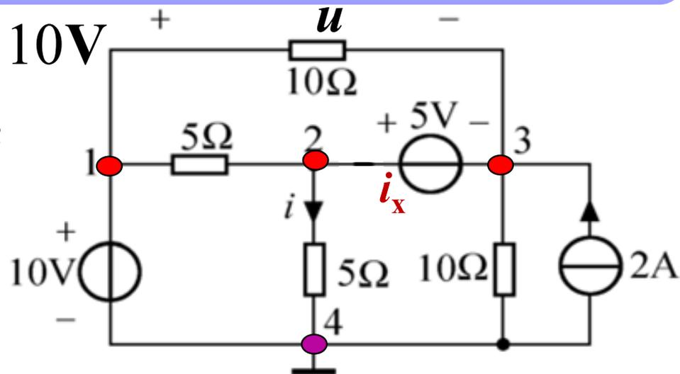
$$\begin{cases} u_{n1} = 10\text{V} \\ -\frac{1}{5}u_{n1} + \left(\frac{1}{5} + \frac{1}{5}\right)u_{n2} = -i_x \\ -\frac{1}{10}u_{n1} + \left(\frac{1}{10} + \frac{1}{10}\right)u_{n3} = i_x + 2 \\ u_{n2} - u_{n3} = 5\text{V} \end{cases}$$
