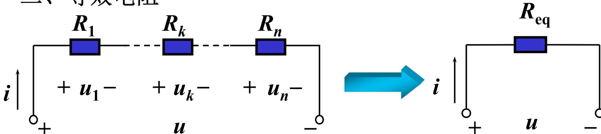
$$R_{eq} = (R_1 + R_2 + \dots + R_n) = \sum R_k$$
